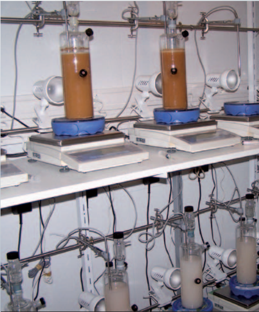
To assess the fermentation performance of the different Lallemend yeast strains and the efficiency of nutrients, a system for online monitoring of fermentation has been developed in close collaboration with INRA Montpellier (thanks to the expertise of the Team UMR-SPO).
